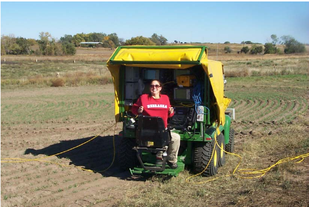
Figure 17. Weather was very pleasant most days with highs in the 70s to 80s and lows around 40. The seismic recording vehicle housed the Geometrics NZC controller and one Geode used to record the vibrator ground force. All data were transmitted to the recording vehicle from the other ten Geodes via ruggedized Ethernet cables. Graduate student Theresa Rademacker of Lincoln, Nebraska, recorded data and performed initial data quality control monitoring of the 240-channel uncorrelated vibroseis data and ground force pilot trace.
