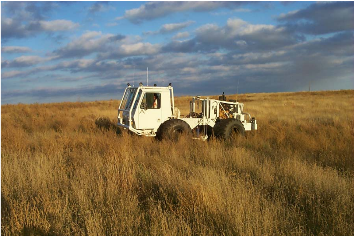
Figure 15. David Thiel operating the IVI minivib2 with GPS tracking and guidance system. A two to four times increase in power was obtained after installation of an Atlas rotary style servo valve in comparison to the factory Moog valve.
