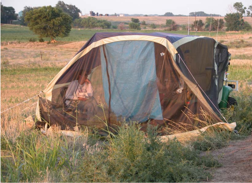
Figure 25. Mosquito netting was draped over the seismograph vehicle to keep the air temperature equivalent to outside air, allow a breeze at the operator station and across the equipment, and keep insects away.
