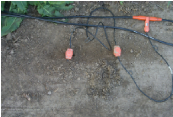
Figure 14 Two 40-Hz high-output geophones
