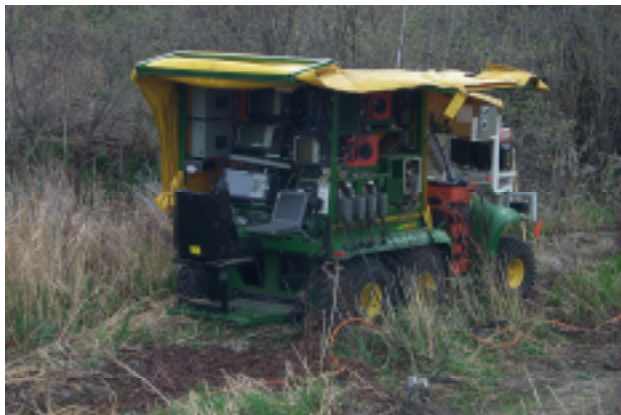
Figure 9. 240-channel Geometrics StrataView with StrataVisor controller mounted on a 6-wheel John Deere Gator.
