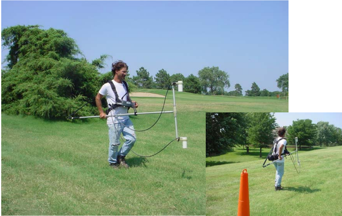
Figure 3. A portable cesium gradiometer G858 was used to measure the total component of the geomagnetic field.
