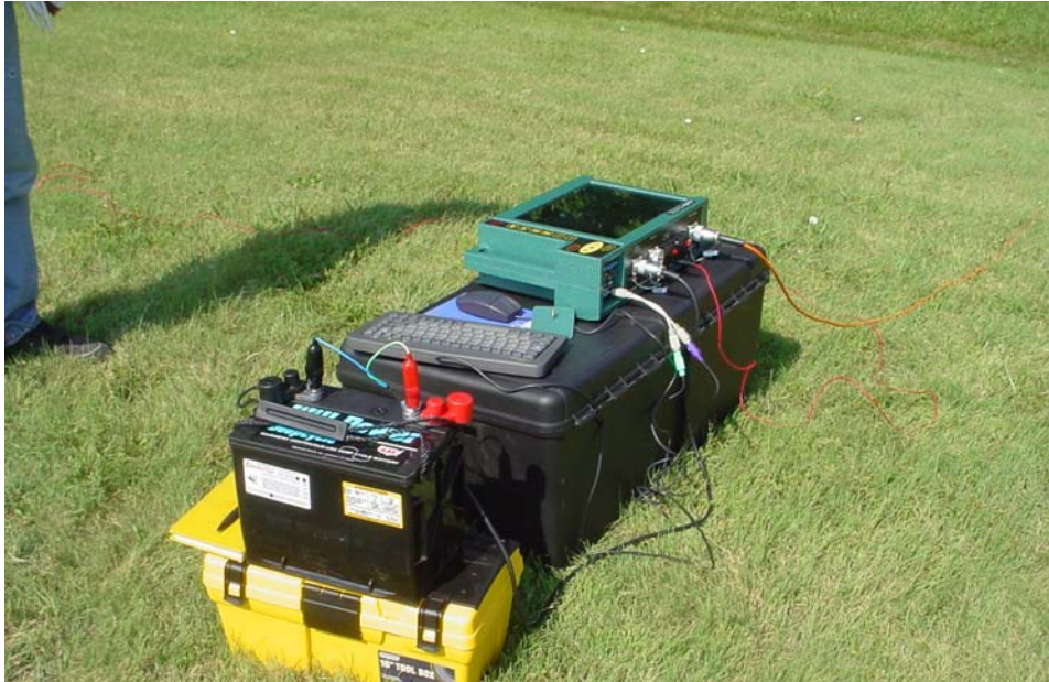
Figure 7a. A Geopen™ E60C multi-electrode resistivity meter was used in ERP survey.
