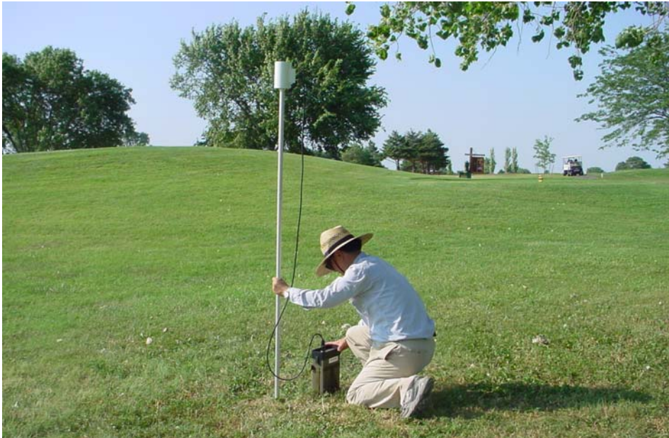
Figure 5. A Geometrics G856 proton magnetometer was used to measure the diurnal changes of the geomagnetic field.
