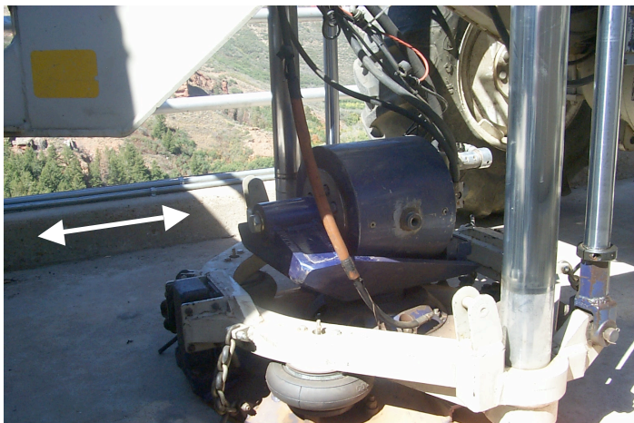
Figure 31. Vibrator mass/baseplate located on dam crest in longitudinal configuration. Arrows here and in Figure 30 show the axis of the vibrator mass.
