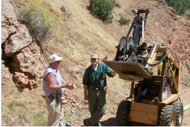
Figure 19. Case loader with RAWD attached to loader arms. Hydraulic power is provided by the loader.
