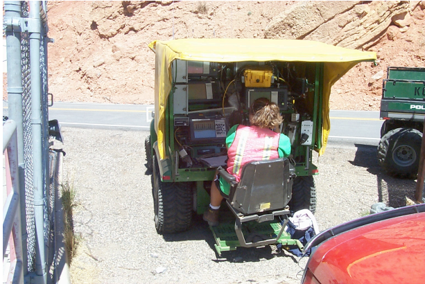
Figure 8. Geometrics StrataView 240-channel seismograph w/NZC StrataVisor controller mounted on a 6-wheel John Deere Gator ATV.
