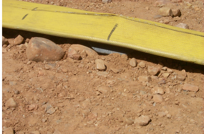
Figure 42. Towed spread along the toe road. The steel shoe on the bottom of the fire hose acts to slice through the loose material to improve receiver coupling. Cobbles and larger gravel would cause the shoe to ride up and degrade the overall coupling.
