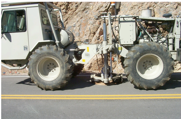
Figure 14. IVI minivib1 in SH mode along abutment.
