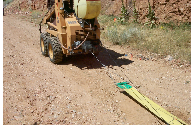
Figure 20. Case loader towing the streamer with cable attached to an electric winch to allow quick changes in source offset.
