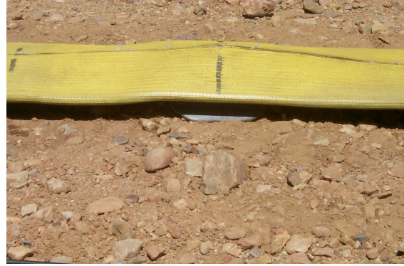
Figure 25. Fire hose and geophone steel shoe. The steel shoe cut through loose surface material and provided a solid ground couple.
