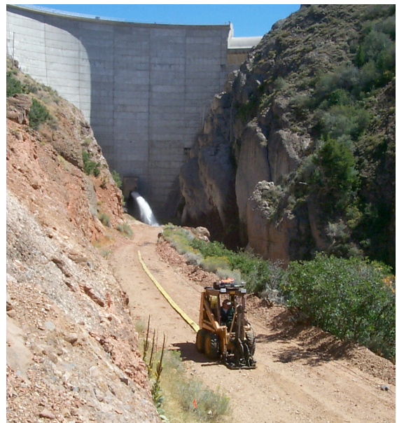
Figure 26. Towed spread configuration for data acquired along the toe line.
