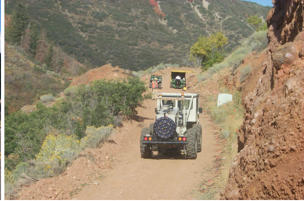
Figure 13. Vibrator setup on toe road with rock ledges both north and south of road. Seismograph vehicle set up to allow vibrator to move past during acquisition. Receivers are along north side of road.
