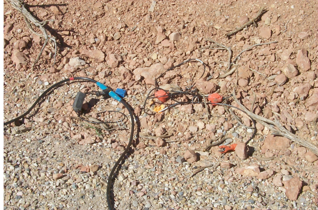
Figure 9. Shear geophone (blue) planted with compressional geophones (red) at a typical location along toe road.
