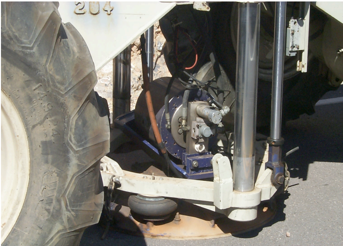
Figure 21. Vibrator pad with mass oriented transverse to line direction and center line of vehicle.
