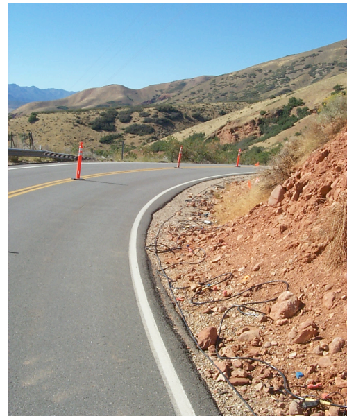
Figure 11. Geophones were planted in loose gravels along the north-road shoulder. Coupling was generally poor and inconsistent.
