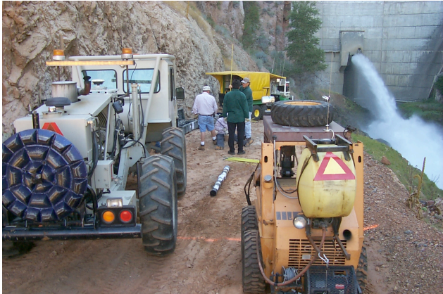
Figure 17. Vibrator and RAWD equidistant from toe borehole. Vibrator was producing shear energy and weight drop was providing compressional.
