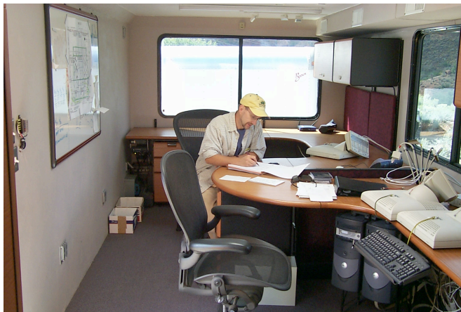
Figure 40. Mobile processing facility on-site and used to perform data quality checks. Three on-board computers and two plotters with Ethernet connections to the seismograph allow rapid in-field data analysis.
