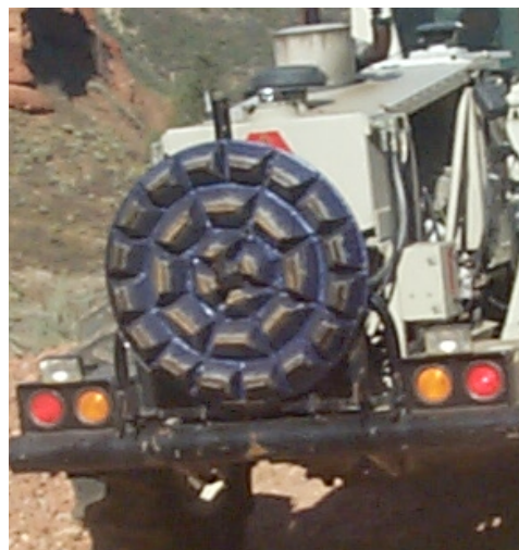
Figure 22. Waffle plate (blue) traditionally used to couple the baseplate to ground surface. Damage and lost coupling precludes its use on paved roads.
