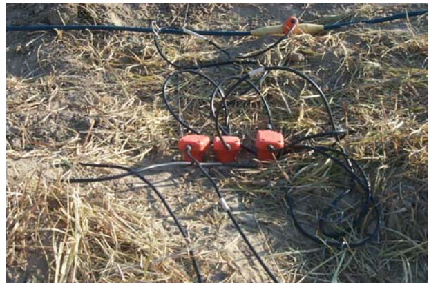
Figure 21. Compressional-wave phones used for through-levee, site 1.
