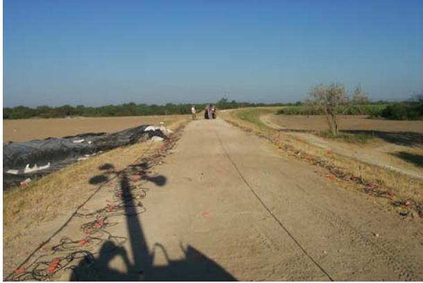
Figure 27. Seismic lines deployed along each side of crest road at site 2.
