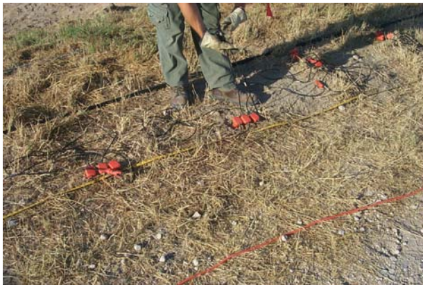
Figure 29. Receiver station spacing was 3 ft.
