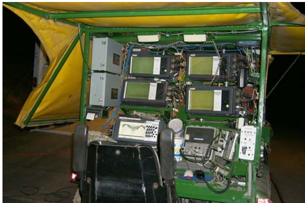
Figure 6. Geometrics 240-channel seismograph mounted in John Deere Gator.
