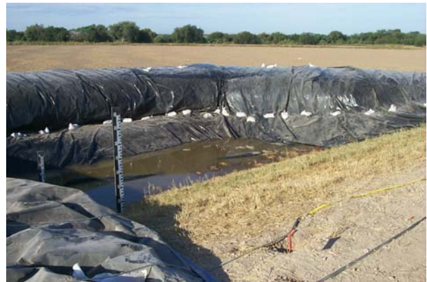
Figure 30. Pond was incrementally filled to simulate rising water from Rio Grande flood.
