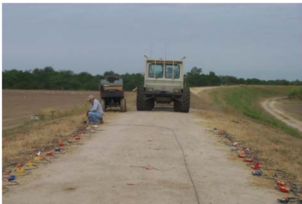
Figure 35. Vibrator on-line and ready to begin dwell experiment at various pool stages.
