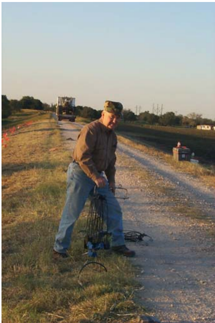
Figure 9. Both compressional and shear geophones were used at each station.
