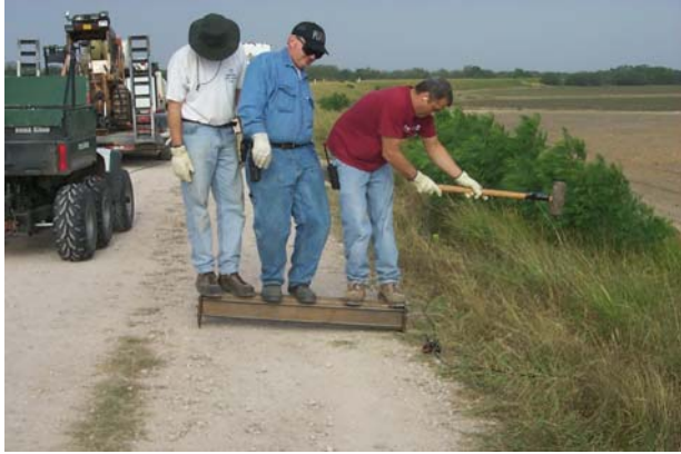
Figure 11. A 1-m-long wood block with steel end plates held down by standing on top of the block was used to generate shear energy.
