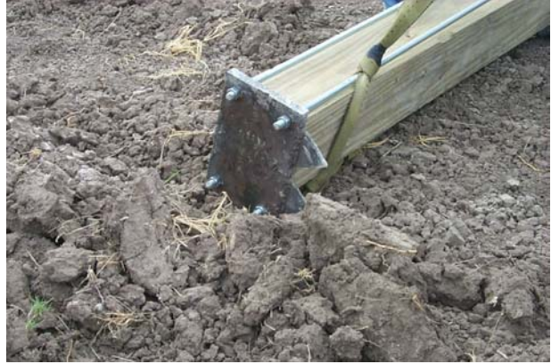
Figure 12. Steel teeth were forced into the ground to minimize source decoupling and sliding along ground surface.
