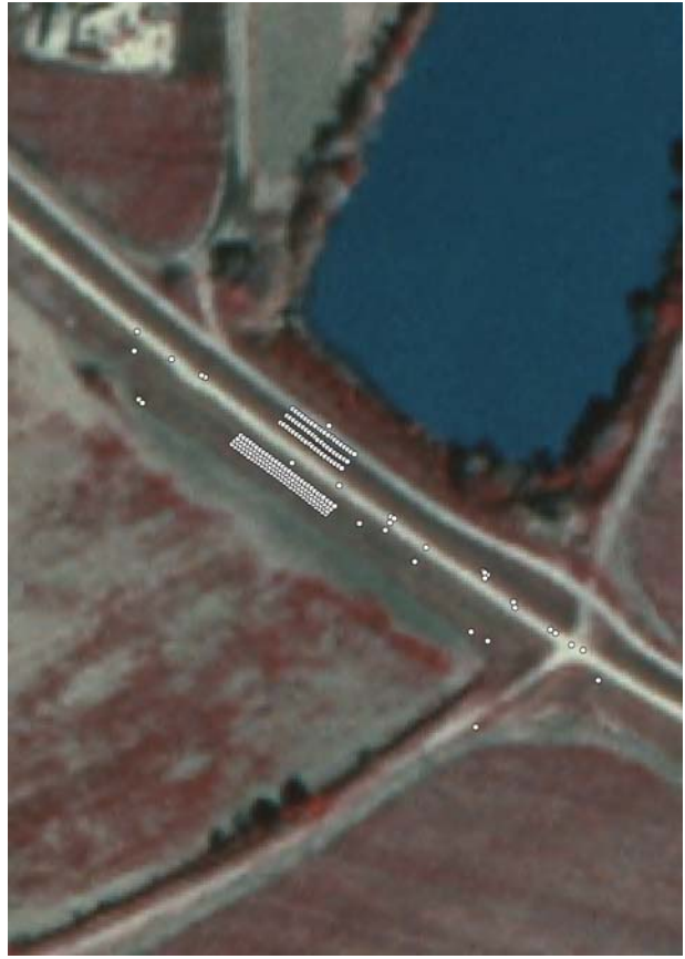
Figure 15. Through-levee receiver and source grids at site 2.
