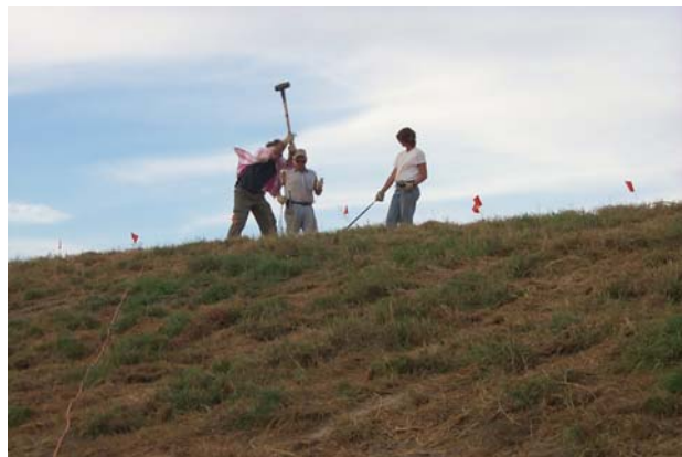
Figure 10. Compressional-wave survey along levee crest road.
