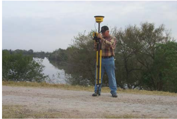
Figure 13. Differential Global Position System (DGPS) was used to accurately locate all sources and receiver stations.
