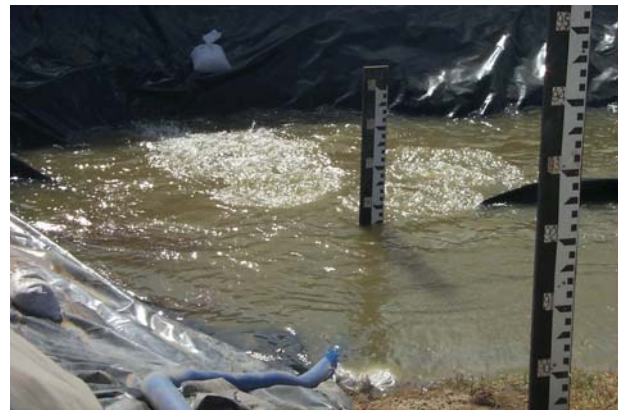
Figure 26. Water pumped into pond at rate consistent with model flood.
