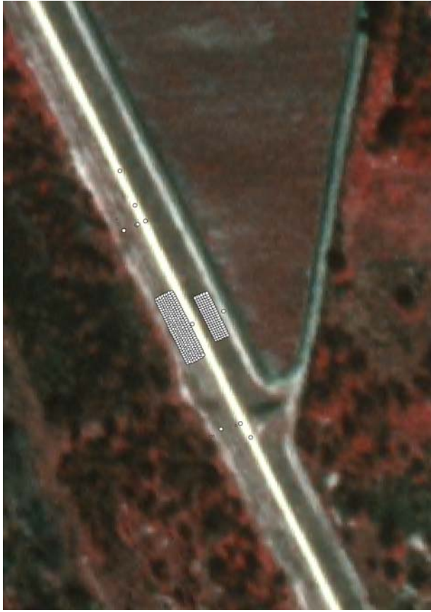
Figure 14. Through-levee receiver and source grids at site 1.
