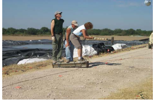
Figure 34. Shear-wave survey during full pool.
