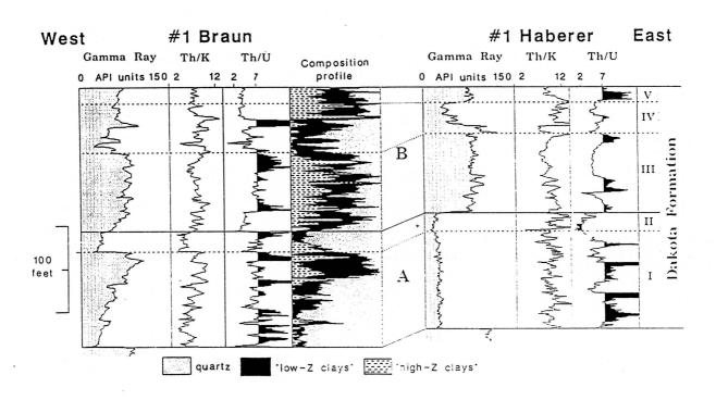
Figure 3. Computed gamma ray, Th/K, Th/U, and RHOMAA-UMAA composition logs for the KGS #1 Braun and computed gamma ray, Th/K, and Th/U logs for the KGS #1 Haberer in the Dakota Formation.
