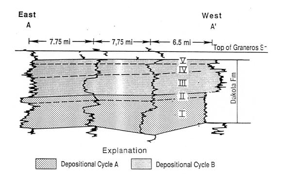
Figure 5. East-west subsurface cross-section, Graneros Shale and Dakota Formation from the KGS #1 Haberer to the KGS #1 Braun.
