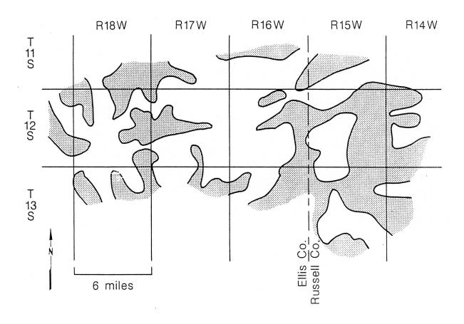
Figure 14. Distribution of sandstone aquifer units deposited in the vicinity of deltas during the Cretaceous Period, middle part of the Dakota Formation. Areas of sandstone accumulation are shown in a stippled pattern.
