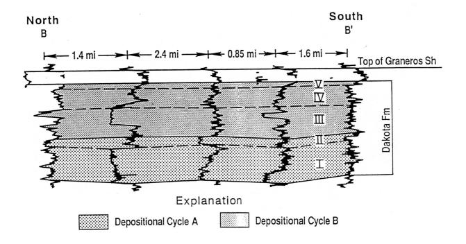
Figure 7. North-south subsurface cross-section through the KGS #1 Braun, Graneros Shale and Dakota Formation.
