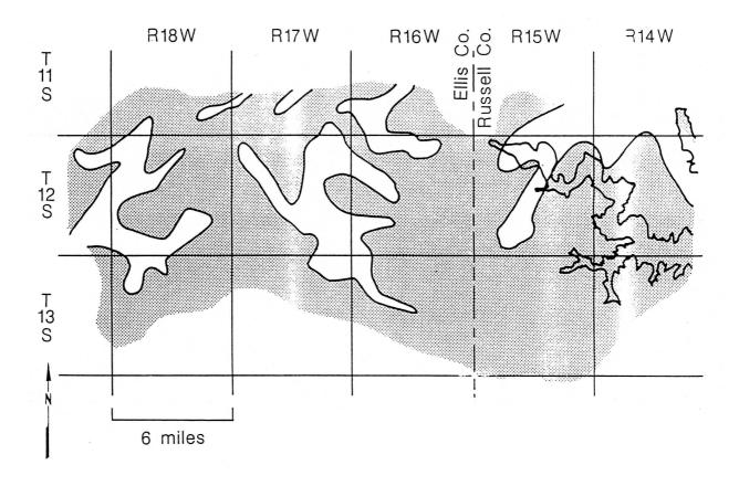
Figure 15. Distribution of sandstone aquifer units deposited in the vicinity of deltas during the Cretaceous Period, uppermost part of the Dakota Formation. Areas of sandstone accumulation are shown in a stippled pattern.
