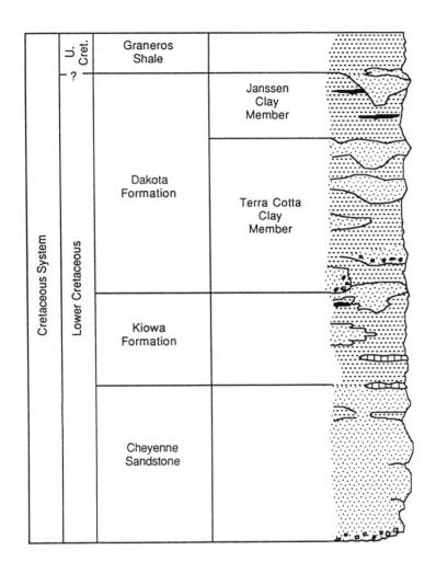
Figure 2. Schematic stratigraphic column showing the distribution of rock types and sandstone aquifers in the Lower Cretaceous rocks.
