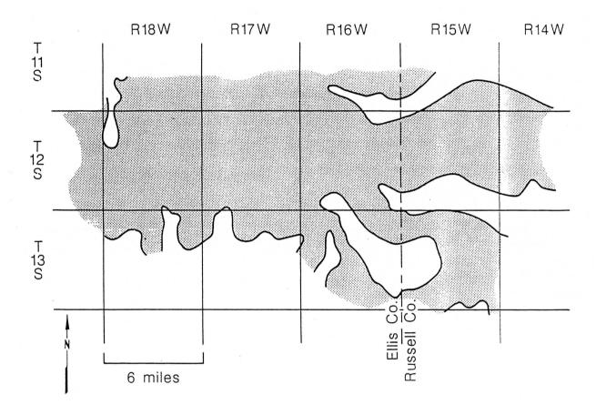
Figure 12. Location of the lower fluvially-deposited (deposition in stream channels) sandstone aquifers in the Dakota Formation, western Russell and eastern Ellis counties. Areas of sandstone accumulation are shown in stippled pattern.
