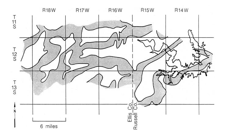
Figure 13. Location of the upper fluvially-deposited (deposition in stream channels) sandstone aquifers in the Dakota Formation, western Russell and eastern Ellis counties. Areas of sandstone accumulation are shown in a stippled pattern.
