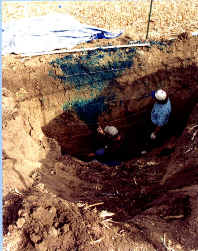
Figure 15. Funnel front pattern from Brilliant Blue dye tracer experiment at site N7.
