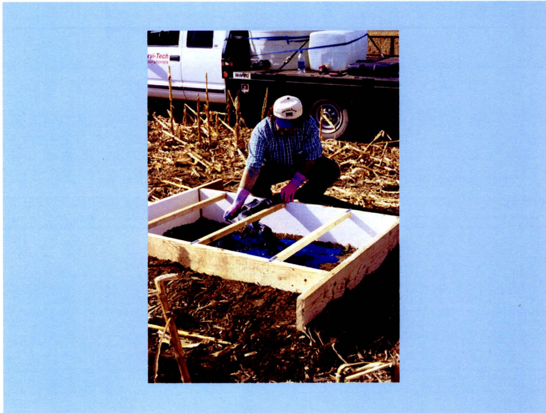
Figure 9. Wooden rectangular frame for flooding the site with dye solution.
