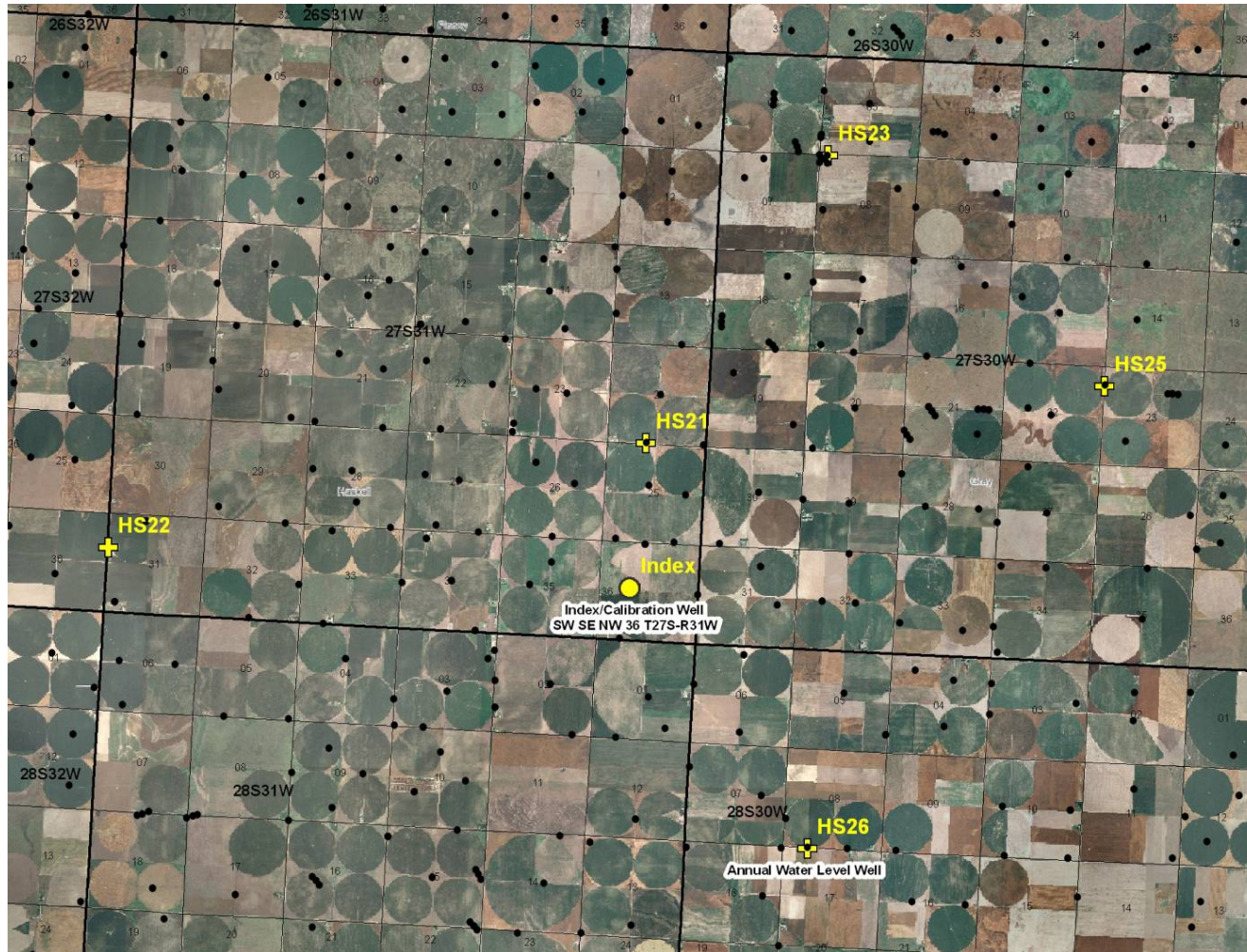
Figure 3.1. Haskell County site area with annual water-level (WIZARD) wells (yellow crosses) and production wells (black dots).
