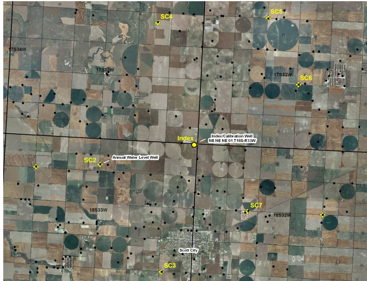
Figure 4.1. Scott County site area with annual water-level (WIZARD) wells (yellow crosses) and production wells (black dots).
