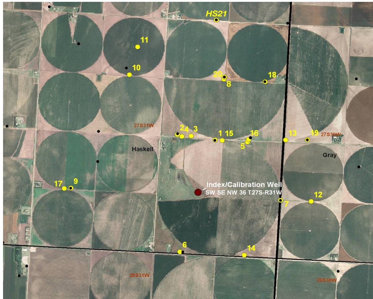
Figure 3.2. Haskell County site area showing wells that KDA-DWR is monitoring (yellow dots) and production wells (black dots).
