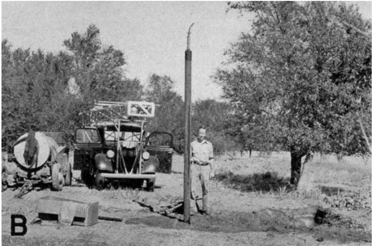
Figure 19. Test well in Meade County State Park, drilled 1939 (head of 17.4 feet above the land surface). Taken from Plate 7b of Frye (1942).
