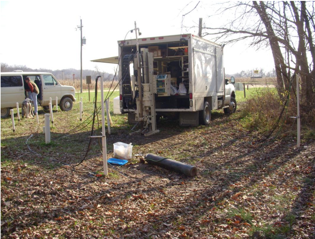
Figure 53a. Geoprobe unit on site for pneumatic 3 second data collection.
