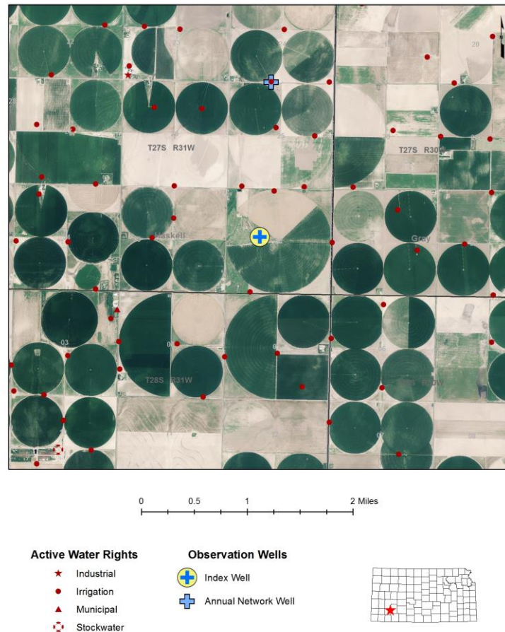
Figure 2—Haskell County site, showing the index well, an additional annual network well, and the nearby points of diversion. Pumping wells that are monitored by DWR are not marked and observation wells monitored by DWR are not shown.
