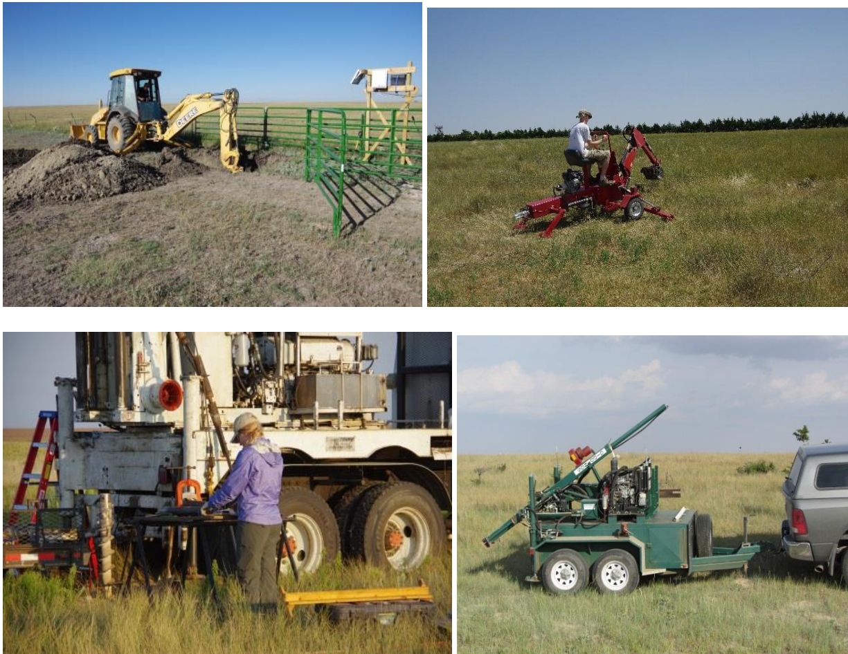
Figure 17. Sub-surface investigations. Trenching was conducted using a locally contracted backhoe and operator (UL), and shallow soil-inspection pits were excavated with a small towable backhoe by Nate Schlagel, as well as by soil probing and hand bucket auguring (UR). Extraction of cores was conducted by the Kansas Geological Survey's Exploration Services section drill crew using a hollow-stem auger system (LL; Kait Salley pictured logging cores), and by using a trailer-mounted Giddings coring machine (LR). (W.C. Johnson)
