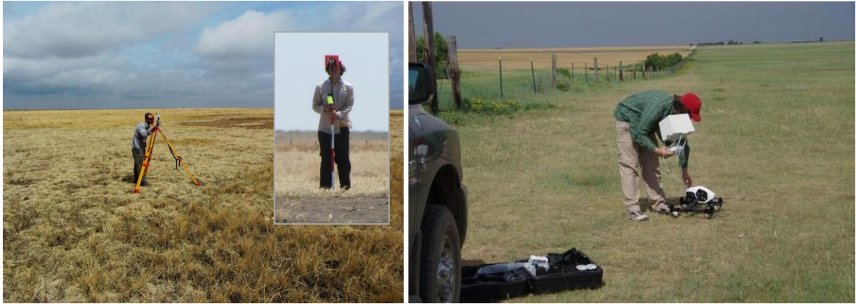
Figure 7. Examples of approaching the field-based characterization of Ehmke Playa. (L) Mark Bowen and Dakota Burt (inset) employing a total station system to establish a datum and map the playa via a series of intersecting transects. (M.W. Bowen); (R) Dakota Burt preparing to launch one of our research sUAS for a photographic mission. (W.C. Johnson)
