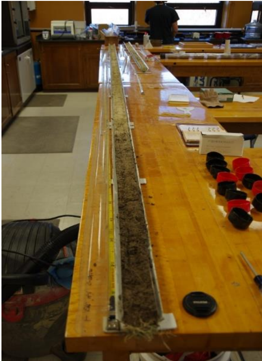
Figure 21. Drill core analysis in the laboratory. The EPC4, the 7.25 m (23.8 ft)-long south bench core, has been opened (view down core) and dressed for description, photography, sampling, and color scanning in the University of Kansas Soils and Geomorphology Laboratory. (W.C. Johnson)
