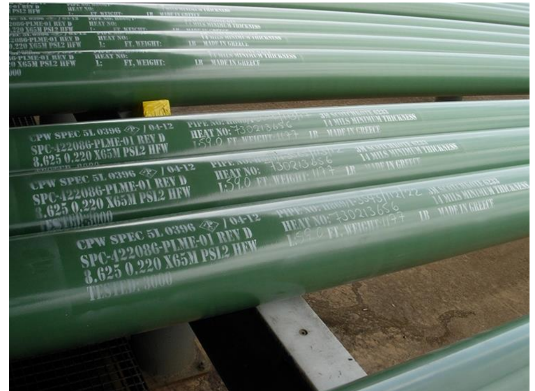
Line Pipe for Coffeyville CO 2 Pipeline
