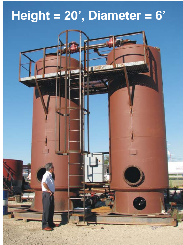
Figure 23: Photograph of the new and larger plant that has been built by American Energies Corporation for installation in one of their low-BTU fields where the wells are currently shut for lack of availability of rich gas for blending.
