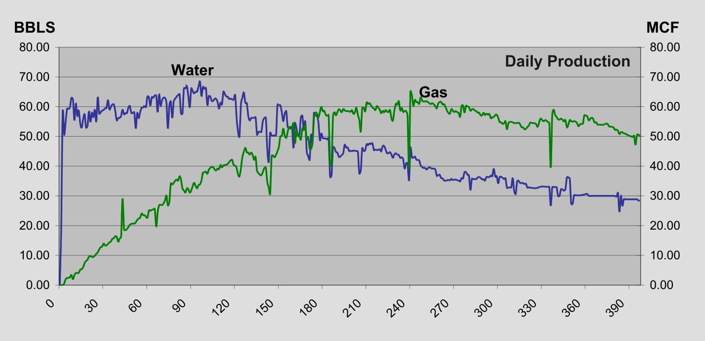
A typical production curve of a CBNG well in Wilson County, Kansas, showing the daily rates of gas and water production. After the well is completed water is produced to reduce the reservoir pressure. The reduction of reservoir pressure leads to the desorption of gas. Unlike a typical gas well, gas rates in a CBNG well increase for a period before they begin to slowly decline.
