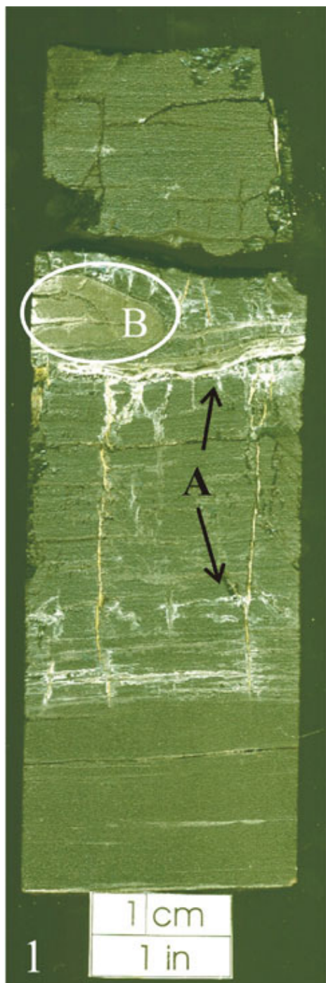
Figure 2.03 - Polished core section showing the coal facies of the Riverton coal. Coal is laminated with variations in lithotypes and macerals. Note mineralization of calcite (A) and pyrite (B) along cleats and laminations. Sample 1 from 850' in the Cooper CW#1 well, 11-T35S-R18E, Labette County, Kansas. Sample 2 from 895' in the Hinthorn CW#1 well, 14-T32S-R16E, Montgomery County, Kansas
