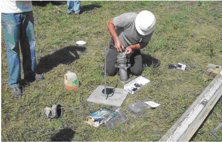
Figure 1.11 Collection and canistering of coal core samples
