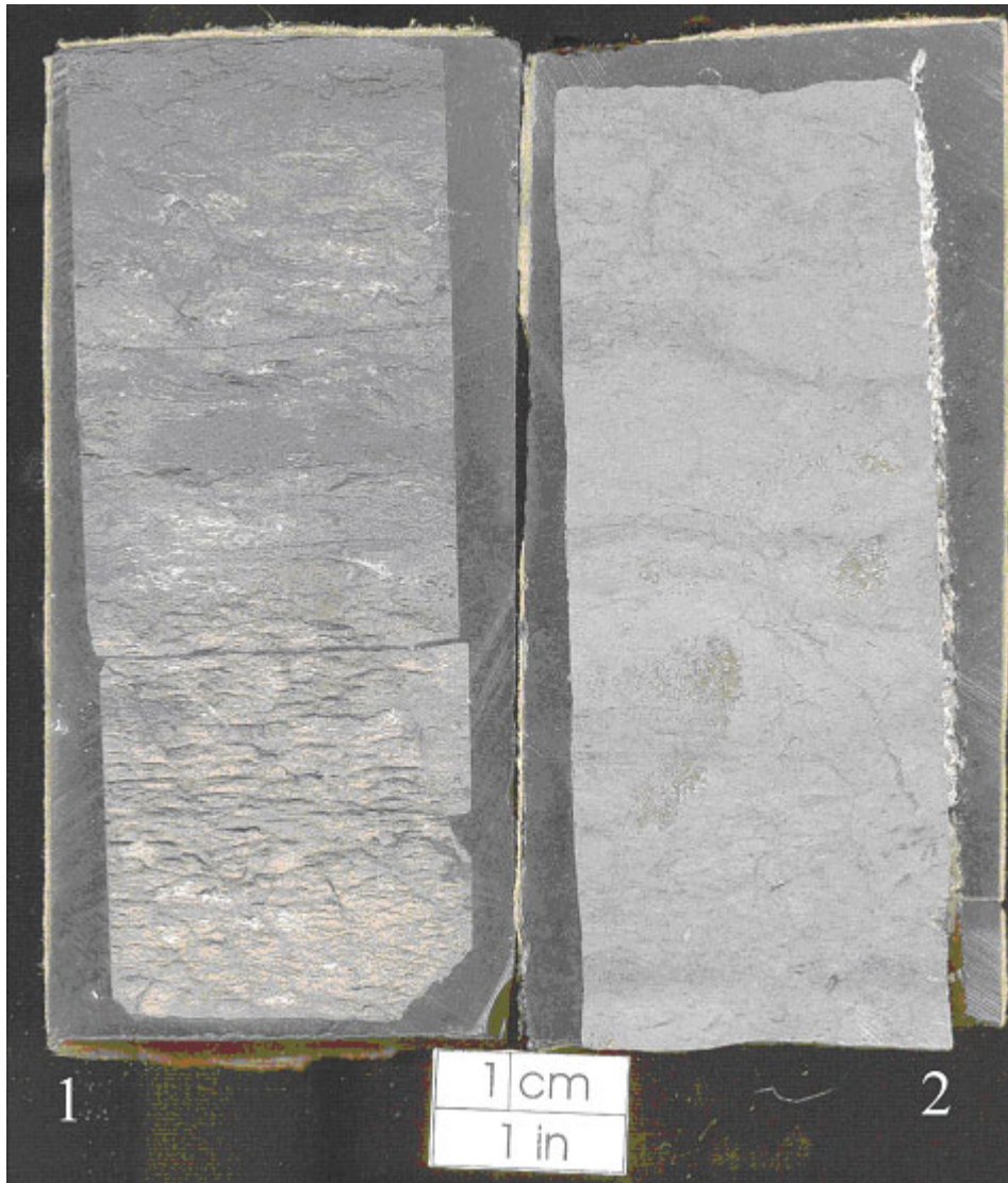
Figure 2.04 - Polished core section showing blocky mudstone facies. Note pedogenic nature and weathered appearance of the mudstone. Soil slickensides are also observed within the blocky mudstone. Sample 1 from 780' and sample 2 from 870' in the Hinthorn CW#1 well, 14-T32S-R16E, Montgomery County, Kansas
