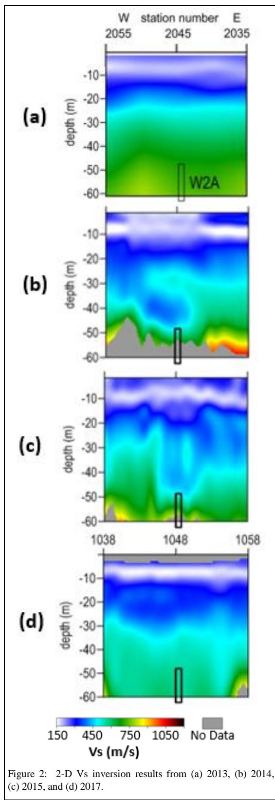
Figure 2: 2-D Vs inversion results from (a) 2013, (b) 2014, (c) 2015, and (d) 2017.
