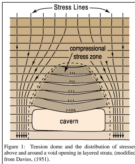
Figure 1: Tension dome and the distribution of stresses above and around a void opening in layered strata. (modified from Davies, 1951).
