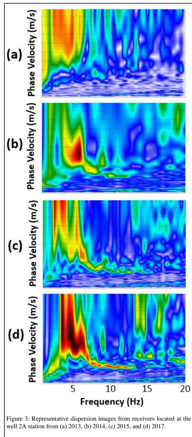
Figure 3: Representative dispersion images from receivers located at the well 2A station from (a) 2013, (b) 2014, (c) 2015, and (d) 2017.
